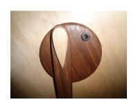
Insert pin into footman retainer. Left for spinning, right for plying
