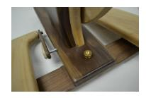
Set body base onto peddle assembly and gently tighten nut
